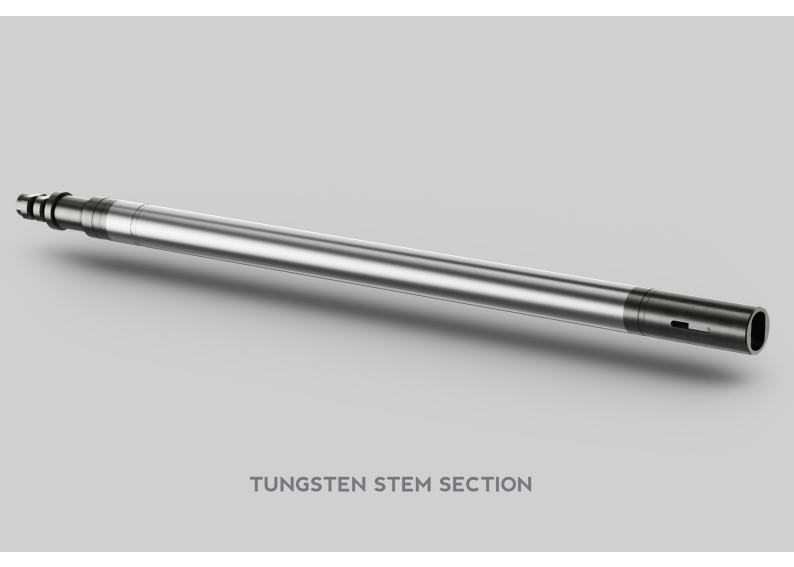
The LiMAR® Tungsten Stem Section is devised to provide the necessary mass required for a wireline toolstring to overcome static or flowing well pressure to enable conveyance in the well.
