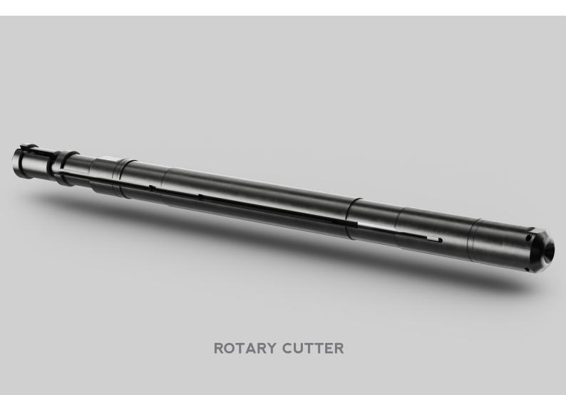
The LiMAR® Rotary Cutter is designed to drop, cut and clamp onto the wireline when a toolstring becomes inadvertently stuck down hole.
