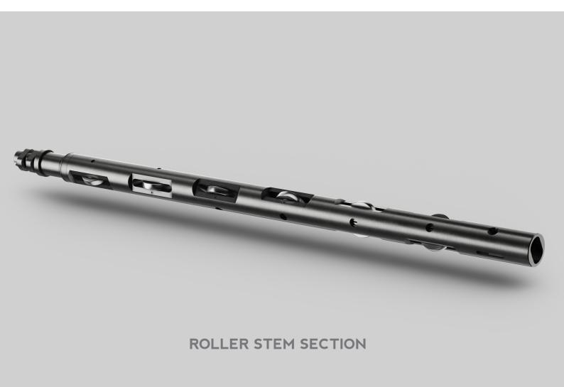
The LiMAR® Roller Stem Section provides the necessary mass and reduced friction required for a wireline toolstring to overcome deviation and the upward-acting effects of well pressure.
