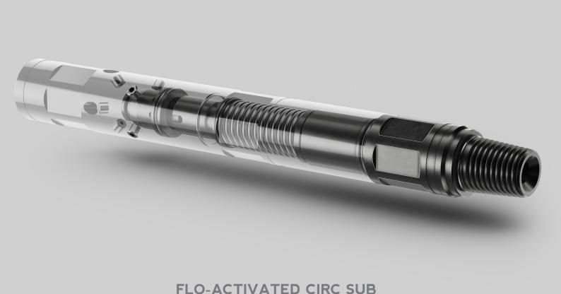
The LiMAR® Flo-Activated Circ Sub can be used in any clean out or milling operation to permit increased flow rate and annular velocity to improve hole cleaning.
