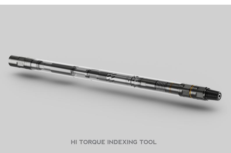
The LiMAR® Hi Torque Indexing Tool allows axial rotation of the BHA to kick over ledges, orientate a fishing BHA or enter a multilateral. The tool is hydraulically actuated, each high flow rate followed by a low flow rate cycle will index the tool through predetermined increments of 30,60,90 or 120 degrees. A high torque ratchet mechanism then fixes the orientation until the next cycle is carried out.
