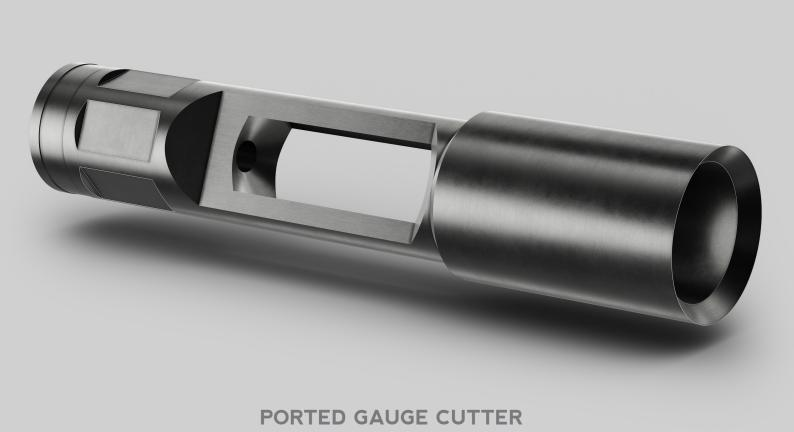
The LiMAR® Ported Gauge Cutter was originally devised to cut and clear deposits from within the tubing. It is now also commonly used as an effective means of drifting the ID of the well during most routine Coiled Tubing interventions.
