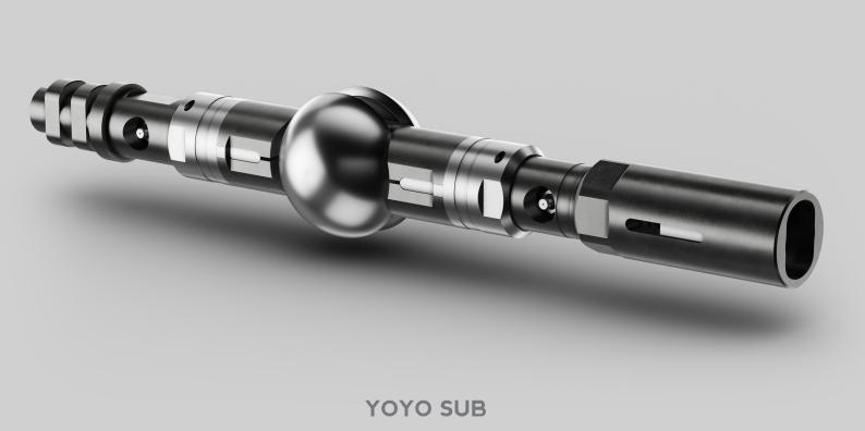
For high angle wells, the LiMAR® YoYo Sub is a compact, rapid-redressable self-aligning system which can be positioned at various points along the length of a toolstring to greatly reduce frictional drag by effectively lifting the string from off of the tubing wall and onto the robust one-piece elliptical roller ball.
